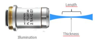
As we use a confocal laser scanning inverted microscope to generate the light sheet, we decided to generate a "scanned" light sheet (also called "virtual light sheet"), one such beam is scanned along a line to create a light sheet, hence many foci are put next to each other.
